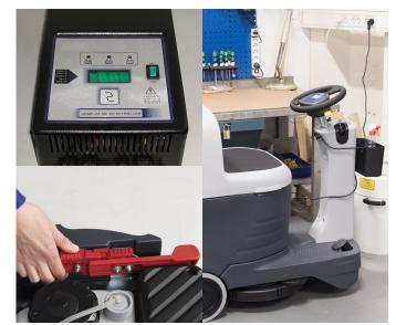
External battery charger 1a. Unplug the Battery charger cable. Reconnect it to the machine.
