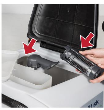
2 Open the recovery tank and check the debris tray and float are clean and working.
