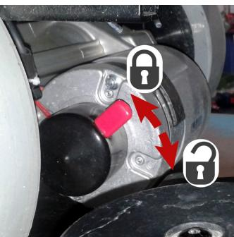
Check if the electromagnetic brake is locking.
