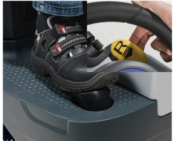
8. Push the drive pedal to start cleaning. Adjust the speed by the pressure on the drive pedal.
